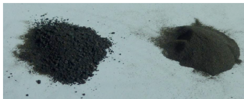
Figure 4. Sieved 100 \mu m JSC-1a. Left oversize, right fines which passed through a 100 \mu m screen.
