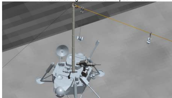
Operational configuration – Mast deployed for payload offloading
