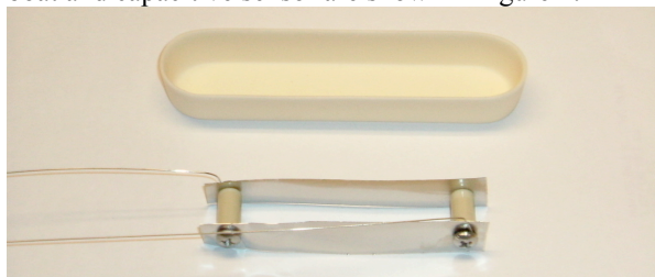
Figure 2. Combustion boat and capacitive sensor. Once the capacitive sensor is placed in the boat, JSC-1A is added until it is level with the top of the boat, with light tamping to level the surface as shown in figure 3. A typical charge is 28.4 grams.
