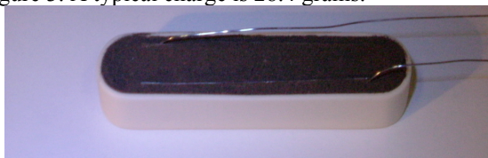
Figure 3. Combustion boat with sensor and JSC-1A. An in-house constructed tube furnace was used, consisting of a Mullite tube 457mm (18") long with and ID of 31.75mm (1.25") with a 304.8mm (12") hot zone wound with Kanthal A1. Multiple mica end zone baffles provide a \pm 5^\circ\text{C} uniformity over the central 203mm (8") at a maximum operating temperature of 1175^\circ\text{C} . The loaded boat and baffles are shown being placed into the tube furnace in figure 4.
