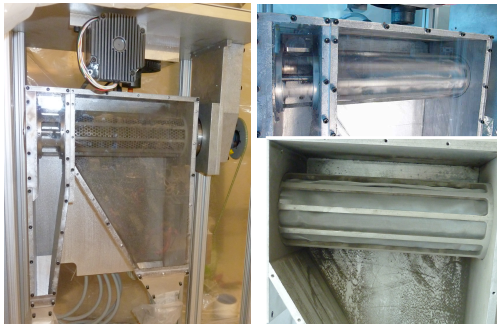
Figure 3. Centrifugal sieve ground testing. Left: 4.6 mm screen. Right: 100 \mu m screen, top video still, bottom post test.
