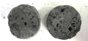
Fig. 4. Cross-section of the product pellet obtained by combustion of Mg/JSC-1A pellet submerged in silica.
